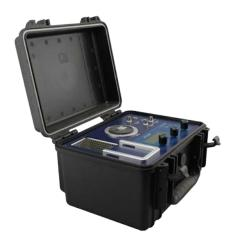
ECS-1028 Portable sensor calibrators are designed to provide on-site sensitivity calibration for acceleration sensors, velocity sensors and displacement sensors(contact types) with frequencies up to 10000 Hz. ECS-1028 Use the comparison method(back to back) for calibration, the automatic closed-loop control is realized through the built-in reference sensor, and the sensitivity curve correction method is used first to achieve the high precision sensor calibration function.
